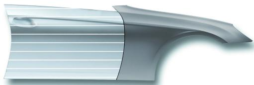
Apply Stadox Basecoat Colorless to adjacent panels. Flash off.
