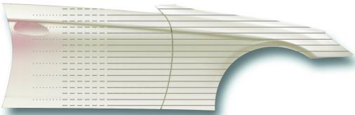
Apply second coat of the effect coat and fade out over the edge of the previous layer into the adjacent panel. Use droplet technique for fading out with reduced pressure.
