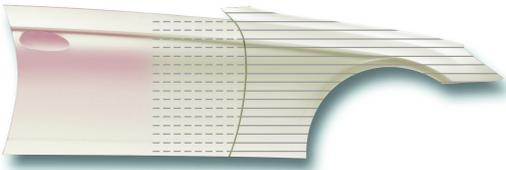
Remove masking and extend with ground colour into adjacent panel. 5 - 10 minutes final flash followed by 15 - 20 minutes at 60-65°C object temperature. Allow surfaces to cool down to normal temperature.
