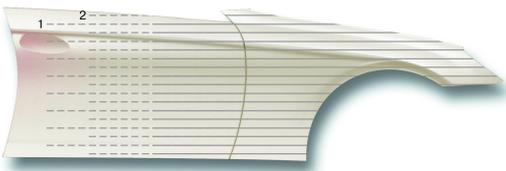
Apply Standohyd Plus Basecoat effect colour to the complete new part and blend-in to the adjacent parts. Spray first coat to the widest area, if needed apply 2nd and 3rd coat with intermediate flash off. Work back from the widest area with staggered overlapping effect coats to avoid a strong halo / visible edge and provide a smooth transition. Start from widest area and work towards centre.
