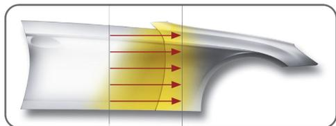
Fade out Standohyd Plus Basecoat with reduced pressure 0.8-1.0 bar, into the wet Standohyd Plus Color Blend 8070 (Work in direction of the arrows)
