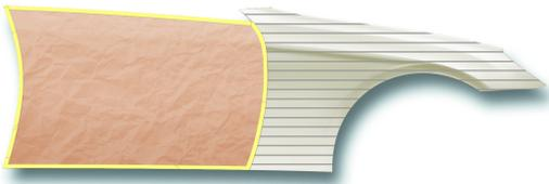
Mask adjacent panels. Apply Standohyd Plus Basecoat ground colour to new panels until complete opacity has been reached.
