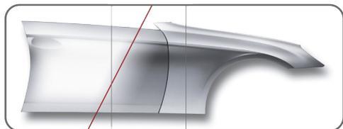
Standohyd Plus Color Blend 8070 is applied in a single spray pass in a wedge shape
