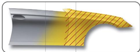
Standohyd Plus Basecoat is applied over the new panel with normal spray pressure to achieve opacity
