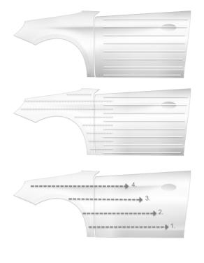
Apply a closed coat of hardened Standoblue Color Blend 8570 / Standoblue Color Blend Slow 8580 (blender +5% Standoblue Hardener 8550) to the adjacent blending area (panel). Do not fade out the blender and apply up to the edge of the panel.
