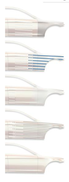
Apply a closed coat of hardened Standoblue Color Blend 8570 / Standoblue Color Blend Slow 8580 (blender +5% Standoblue Hardener 8550) to the adjacent blending areas, avoiding the extreme edges of the panel.
