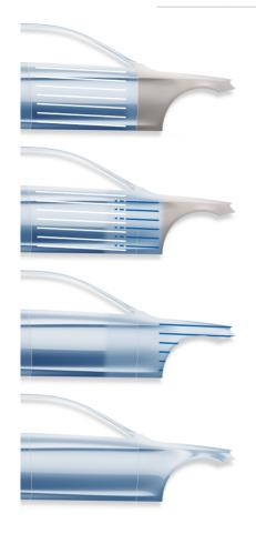
Apply Standoblue Color Blend 8570 / Standoblue Color Blend Slow 8580\* to the surrounding fade out area or adjacent panels with thin closed coats. Do not allow Standoblue Color Blend 8570/8580 to flash.
