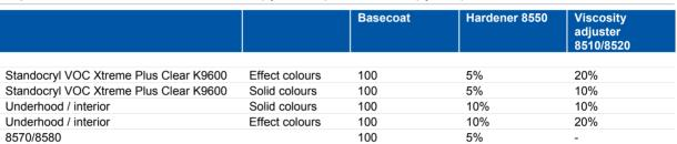
Standoblue Basecoat has the ability to be hardended with Standoblue Hardener 8550 for use in multi-toning, 3-stage ground colors, underhood/interiors and for general application where the basecoat requires to be hardened. The table illustrates the main details, this can also be found in Standowin when preparing the colour ready for use. Standox Demineralized Water 8000 can be added for application in lower humidity and warmer climates.
