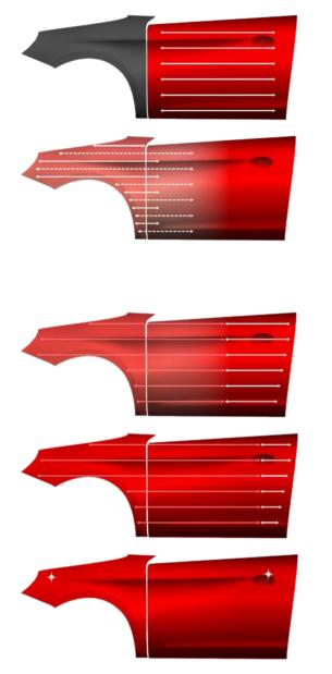
Prepare the repair panel and blending panel according to respective TDS of the Filler and the Standox Basecoat quality being used. Sand the Filler with P500-P600 by machine. Sand the blending area with P1000-1200. Clean surface sufficiently prior to application of the respective Standox basecoat quality.
