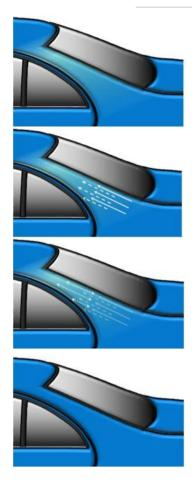
Sanding the fade-out area and the transition to the intact old paintwork, e.g. with 3M Trizact P3000 Fine Finishing Disc or similar abrasives from other suppliers.
