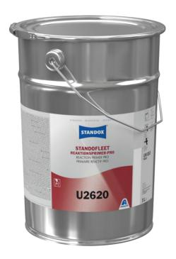
The Standofleet Reaction Primer Pro U2620 is a newly developed zinc chromate free 2K Wash Primer based on polyvinyl butyral especially for the needs in the commercial vehicle and bus sector. Due to its passivating effect, it is particularly suitable for painting aluminum and stainless steel.
